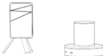
Notice: When the scanner is placed vertically, the calibration board should also be placed vertically.
